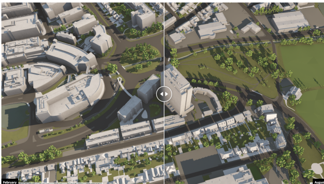
The images below show a comparison between the shadowing caused by the Image Tower in February and August.
